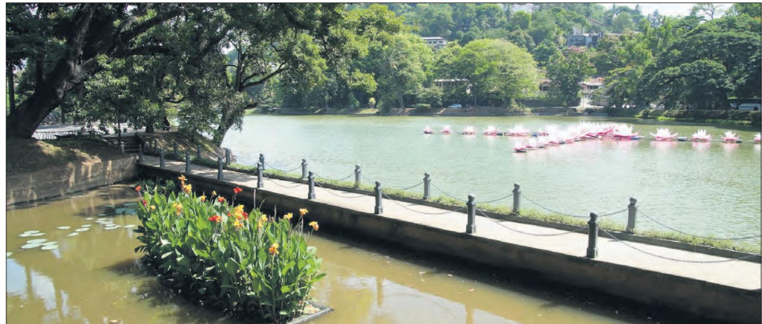
Three plots of “floating wetlands” (above, foreground) were installed to filter out pollutants and silt at an inlet to Kandy Lake in central Sri Lanka. Eventually, 100 of them will be installed. Such wetlands are also used elsewhere in the world, including Singapore and the United States. ST PHOTO: LIN ZHAOWEI
